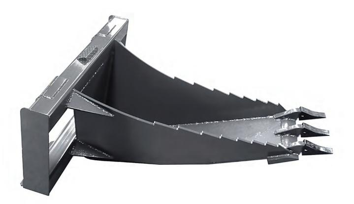
Our X-treme Stump Bucket is made from 1/2" top quality steel plate and features a 1" cutting edge with replaceable teeth. It has a curved bottom, giving you more leverage when prying up rocks and stumps or digging in harder ground. The X-treme Stump Bucket is a full 12" longer than our Heavy Duty Stump Bucket, which allows you to dig much deeper.
