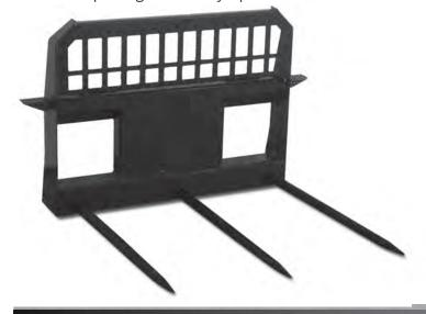
Our X-treme High Back Hay Spear is designed to increase your leverage and safety when rolling the bail back towards the cab. Hay Spears easily move bales of hay with a quick hook up on your skid steer or tractor. Euro style and John Deere mounts are available.
