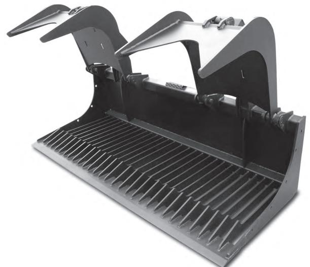
Our X-treme Rock Grapple is great for sifting through dirt in order to remove rocks. With the tines set at 2-1/2" apart, you pick up most everything but the dirt. You can also pick up large rocks, logs, brush or just about anything else by use of the grapples. We use twin 2" bore by 10" stroke cylinders rated at 4,000 psi on all of our grapples.
