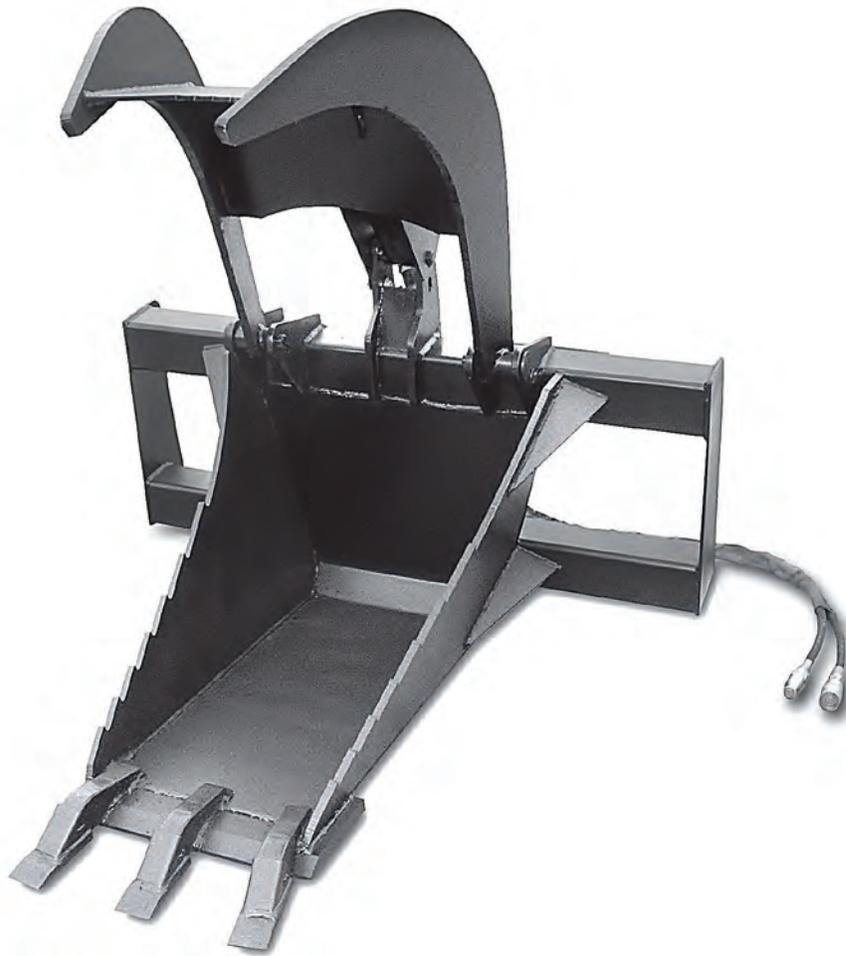
Our X-treme Stump Grapple is made from 1/2" top quality steel plate and features a 1" cutting edge, replaceable teeth and a 3/8" hose. Not only are you able to dig out stumps, you are able to carry them away afterwards. No need to have another attachment for loading the stump into your dump truck, or moving the stump to a burn pile.
