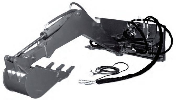
Our X-treme Swing Arm Backhoe is an excellent tool for digging ditches, removing stumps and digging footings. It uses an electric over hydraulic control to operate both the bucket and swing cylinder from one auxiliary valve on your machine. This allows a 110 degree swing right or left.
