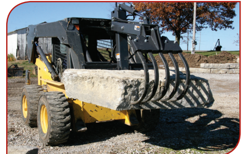
Grabbing and building retaining walls is easy, even with large cut stones or blocks.
