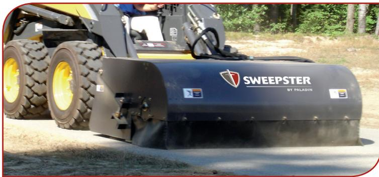
**Sweepster's SSL Collector Sweeper - Hydraulic Drive (SB Hopper Broom & Cold Planer Special)**, by Paladin, handles light and heavy-duty clean-up in construction, municipal and industrial applications. Features bi-directional brooms that sweep forward to pick up dirt and can reverse to sweep in tight areas. Direct-drive bush motors eliminate chains and sprockets.
