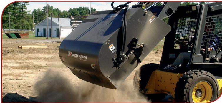
The Cold Planer Special is specially designed to clear heavy millings from cold planer operations. Material is quickly and efficiently collected into the hopper for optimal production and clean-up.
