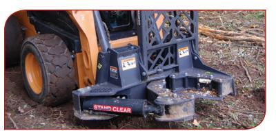
Bradco Tree Shears, by Paladin, are designed for shearing trees up to 10 inches in diameter. A sturdy push bar directs the tree's falling direction. A 4-inch diameter cylinder controls the shear action.
