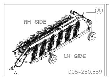
As regards the indicating of right/left, they are understood to be attributed observing the machine from point A (behind the machine) looking forward.
