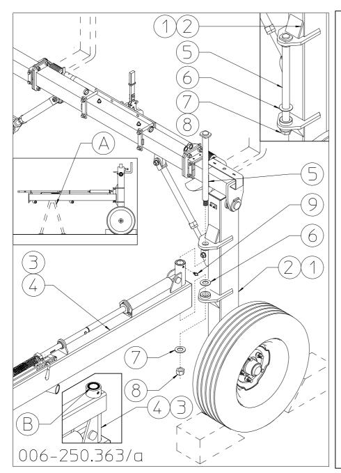
Check that manufacturer has assembled on the vertical supports 1-2 (RH-LH) the pins 5, spacers 6, washers 7 and nuts 8 that you will use for assembly in the order in which you find them assembled.
