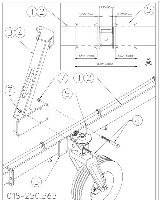
Attach the opening arms 3-4 (RH-LH) to 1-2 sections by of the means counterplates 5, bolts 6 and nuts 7. In box Α the theoretic measurements are given for the assembly of arms 3-4 and counterplates 5. At this stage do not fully tighten nuts 7, because when the cylinders are attached (see step 23) it may be necessary to move the arms 3-4 and counterplates slightly forward or backward to allow the correct installation of the cylinders.
