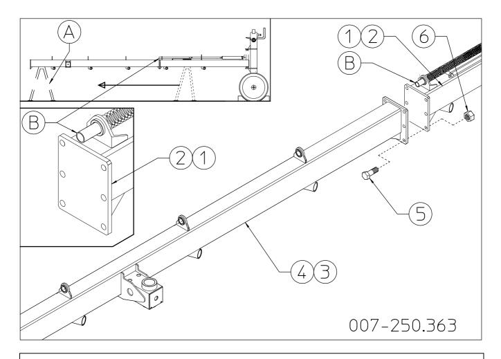
Tube B serves to hold together the spring and the other assembled parts, and it must be removed when the rake wheel lifting pipes are assembled (see step 12).
