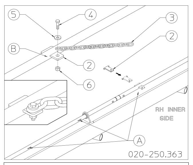
Insert brackets 2 in the slots A in all the pipes (RH-LH). Attach the chain 3 at all the brackets 2 using the bolt, washer 5 and nut 6.
