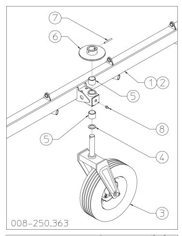
Insert the nylon bushings 5 into the openings in sections 1-2 (RH-LH). Place spacer 4 on the pins of the wheel units 3. Insert the wheel units 3 into the openings in sections 1-2.
