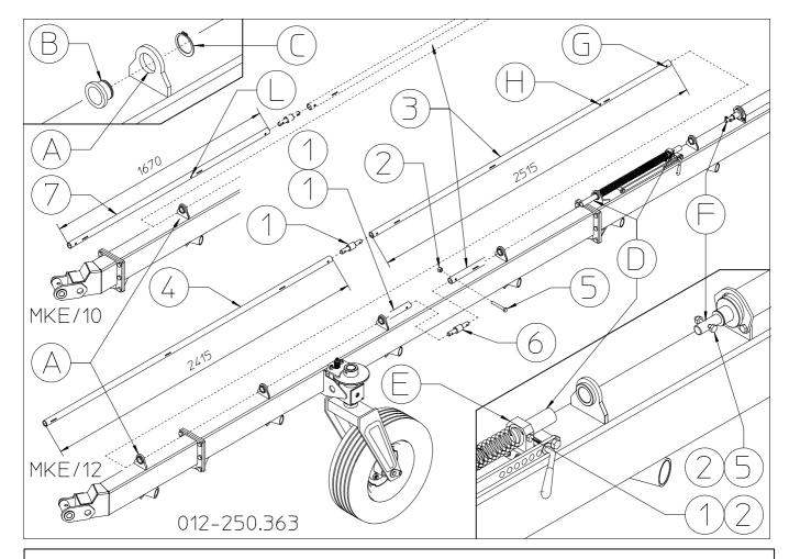
Check to make sure the manufacturer has correctly secured the bushings B with retaining rings C on brackets A on all the RH and LH sections.
