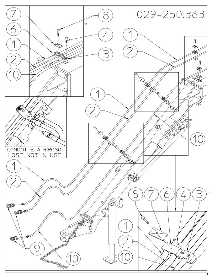
Continue to secure hose 10 with collars 3 and screws 4. Continue to secure hoses 1-2 with collars 6, clamps 7 and bolts 8.
