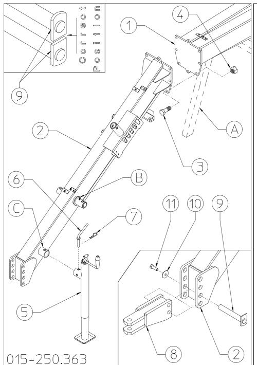
Carry out this operation very carefully and with suitable lifting equipment because the drawbar 2 is heavy and Weight bulky. 60kg/132lbs plus the preceding drawbars. First of all check to make sure the manufacturer has applied the bushings for the safety arms on seat B.
