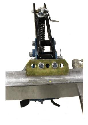
Attach the wheels to the front of the tool bar. The wheels may be located directly behind the tractor tires. They may be located in other positions as well. Some units are set up with the wheels directly in front of the outboard tillage heads. For wide machines this may not be practical. If you are working in raised beds, the wheels will typically be located in a furrow row. There is no right or wrong position for the gauge wheels!
