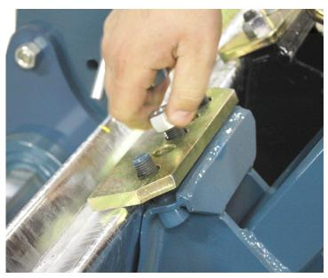
15. The completed three point hitch will resemble the picture below. The top tube has been installed and secured with clamp plates. The last step in assembling the three point hitch is to insert the square plastic caps into the top tube.
