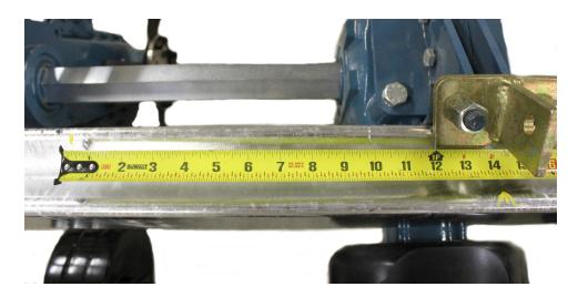
Hitch brackets are secured with clamp plates and hex nuts. Note that the tool bar design allows for elements to be moved on the tool bar as needed and front side and back side elements can slide past each other.
