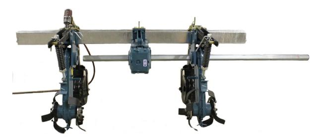
10. One helpful hint before installing the hex shaft is to install one of the outboard locking collars on the hex shaft before pushing the hex shaft through the elements. This will ensure that the locking collar is in place in case you manage to deform the end of the hex bar by pounding on it!
