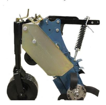
13. Install the PTO shaft cover to the front of the gearbox. At this point your machine should look something like the picture below. The next step is to install the three point hitch.
