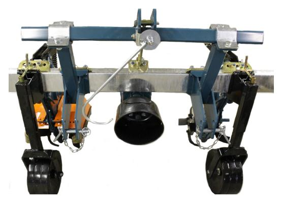
18. Assemble the shielding to the desired width. The shielding comes in three sections - a center section, a right hand side, and a left hand side. It is easier to bolt the shielding together before attaching it to the tillage head. When the shielding is assembled, hook the front shield hooks over the rod shaped bracket on the front of tillage head, and slide the rear of the shielding into the U-shaped support on the rear of the tillage head.
