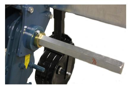
12. Install the guard plates at each end of the tool bar. If the hex bar is centered correctly there should be adequate clearance between the end guard and the hex bar.
