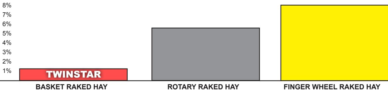
Field test conducted by an independent farm in 2004 measuring the percentage of contaminants in raked hay using the following comparable width hay rakes: 5-Bar 30' Basket Rake, Rotary Rake and Finger Wheel Rake. Results vary due to equipment settings and field & crop conditions.
