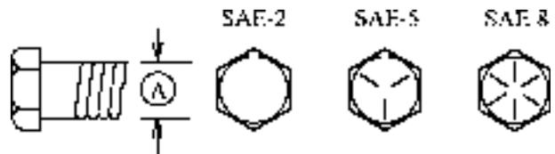
Torque figures indicated above are valid for non-greased or non-oiled threads and heads unless otherwise specified. Therefore, do not grease or oil bolts or capscrews unless otherwise specified in this manual. When using locking elements, increase torque values by 5%.
