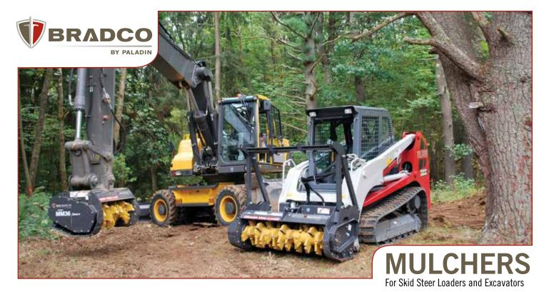
Bradco Mulchers, by Paladin, shred up to 12" diameter hardwood trees using a patented tooth design. Each tooth has a cross bar the full width of the tooth to help keep proper cutting alignment during operation.
