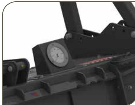
On-board pressure gauge easily viewed from operators station to monitor system pressure (N/S for excavator only models)
