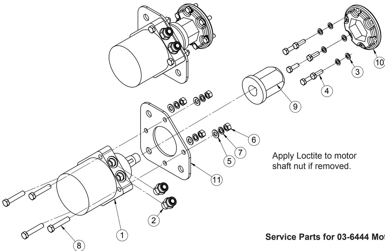
Apply Loctite to motor shaft nut if removed.
