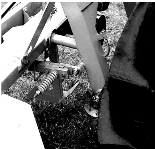
Fig. 8. Safety breakaway device
