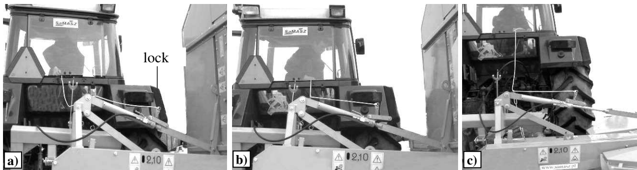
Fig. 17. Mechanical lock of hydraulic lifting function
