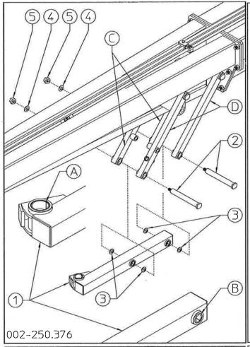
First of all check to make sure the manufacturer has applied the bushings A (two) and bushings B (two + two) to the seats on support 1. Next attach support 1 to the seats on RH supports C and LH supports D using pins 2, shims 3, washers 4 and nuts 5. At this point the nuts 5 (including nuts 6 in the preceding step) can be fully tightened.
