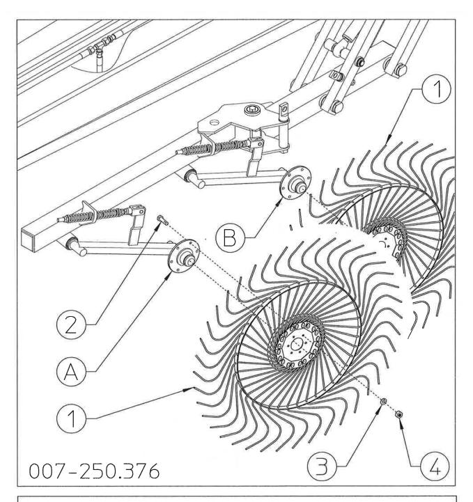
Note: The rake wheels are both RH. Attach the rake wheels 1 to hubs A-B on the arms using bolts 2, washers 3 and nuts 4.
