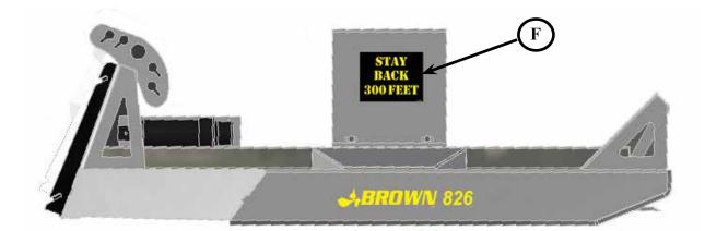
Safety Decals (All Models) Safety decals must be positioned as illustrated below. Use this diagram to correctly identify missing, damaged, or illegible decals for replacement.
