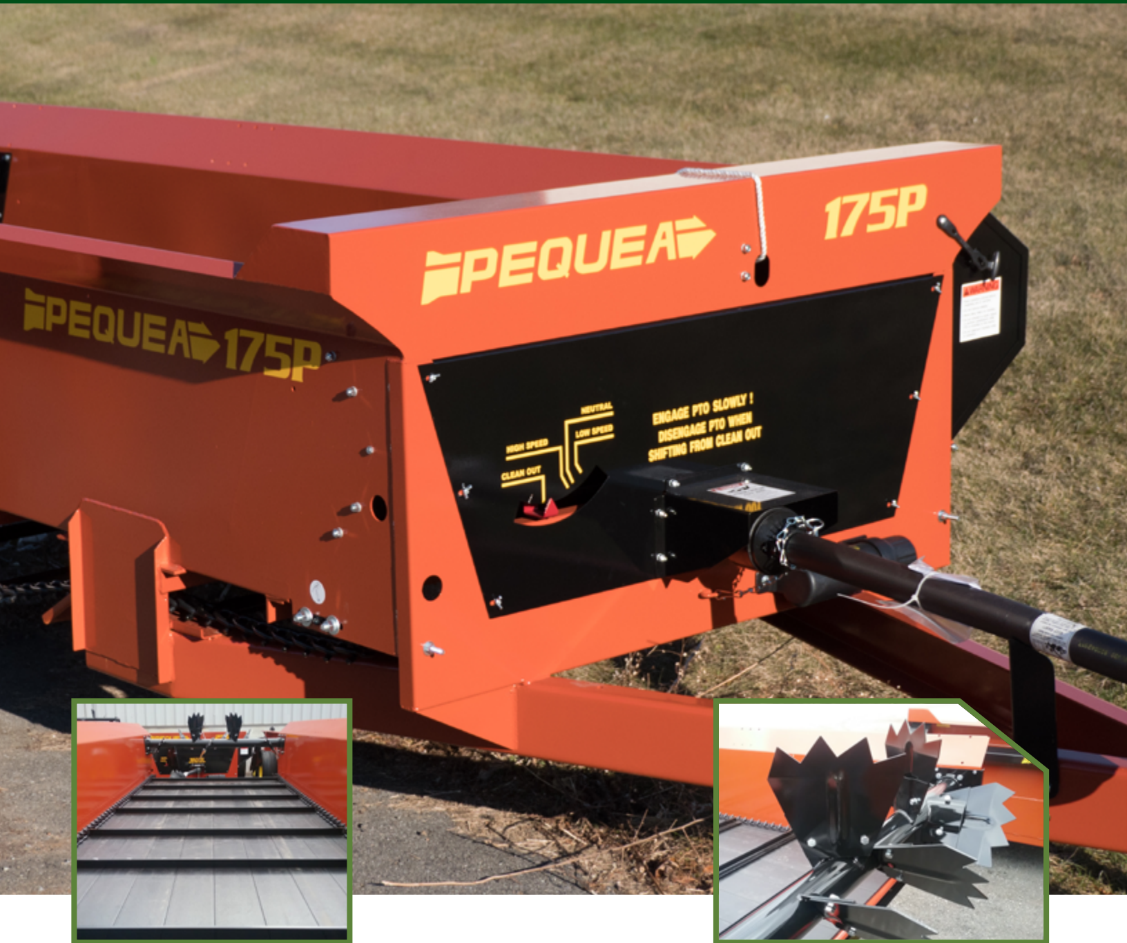
The poly floor helps prevent freezing and never wears out.
