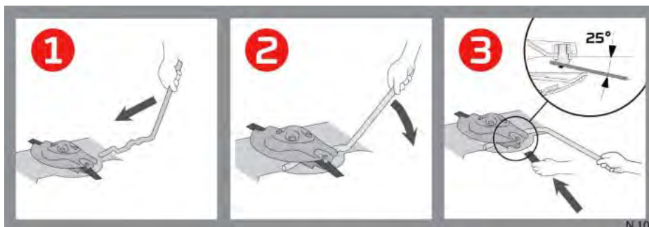
Fig. 22. Quick replacing of the knives with mounting lever
