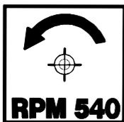
10) Shows the direction of rotation of the power takeoff and the maximum number revolutions.
