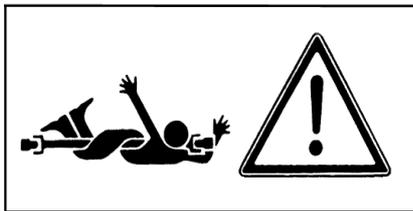
8) Indicates that it is dangerous to touch the cardan (P.T.O.) shaft. For all the other information regarding the cardan shaft, see the use and maintenance booklet specifically for the cardan shaft which, together with this manual, makes up the documentation on safety, use and maintenance of the machine.
