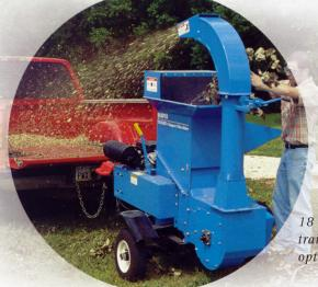
18 HP Honda engine powers trailer mounted model with optional blower attachment.
