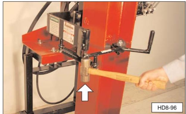
9. Install Lynch pin to secure swing arm to the safety arm frame.
