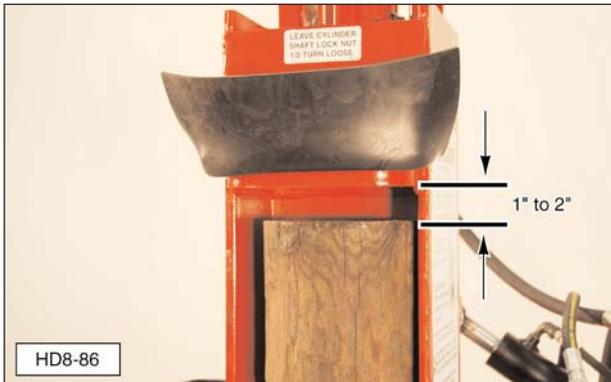
17. Close safety arm frame (I2) to secure the post (the adjustable roller assembly keeps tension on the post while it is being driven).
