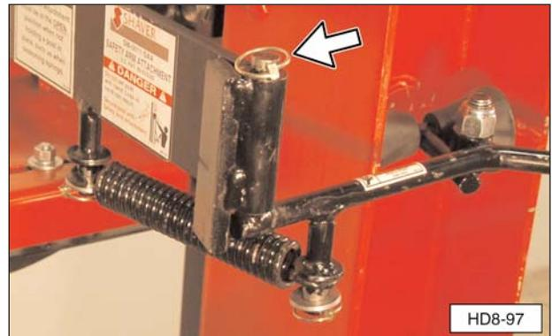
10. Verify the swing arm handle opens against safety arm frame (I2) stop bracket and closes against back wall of drive ram (A1) I-beam.
