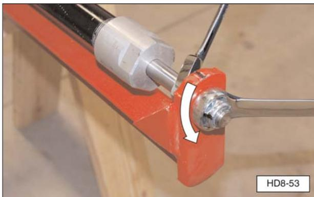
Loosen Lock Nut (C4) 1/2 Turn After Tightening.
