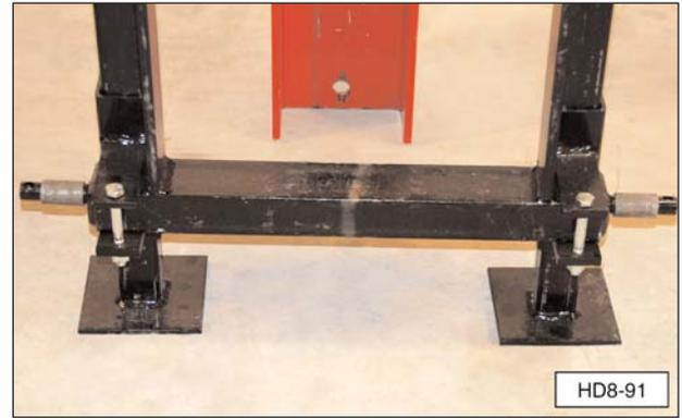
3. Raise or lower the stabilizer legs to allow drive ram I-beam full contact with the ground. Make sure the Post Driver is stable.
