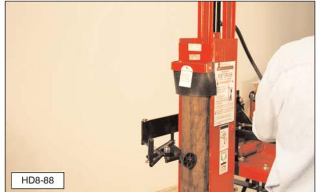
19. Squeeze control valve safety lever (G7) and push control valve lever (G5) to release the drive ram and create impact.
