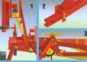
Sitrex Flex-Wing finishing mower is fitted with a tierod system that allows mower's oscillation during working while in transport position this tie-rod system automatically keeps the side mowers in vertical position.
