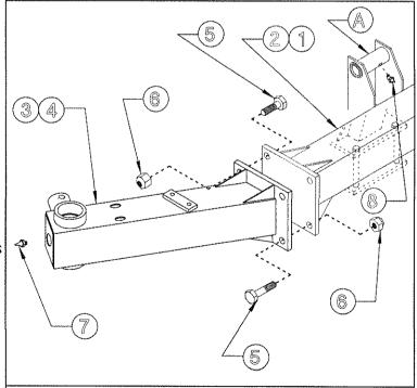
Item 8: 16/14 grease nipples  $M6x45^{\circ}$   $(1/4"x45^{\circ})$
