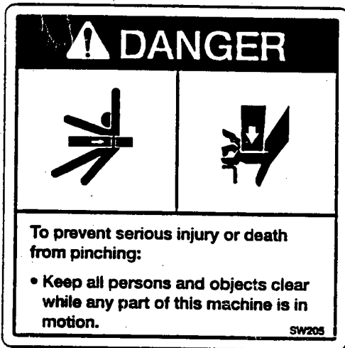
DANGER! PINCH POINTS PART #40149 (2 req'd)
