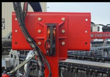
SLIDE TUBES WITH 3 BASKET POSITIONS FOR OFFSETTING BASKETS
