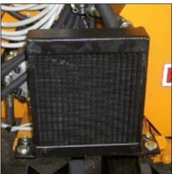
Oil cooler with thermostat (optional TA32).
