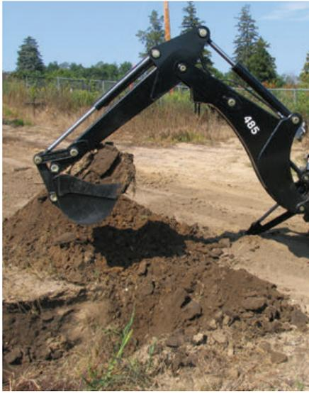
Several classes available depending on desired weight & digging force. 180° bucket rotation and swing arch. Heavy-duty construction grade available for heavy-duty applications. Equipped with cushioned cylinders.
