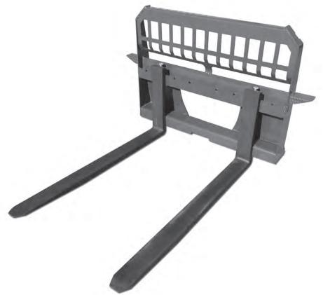
Anyone that owns a skid steer should have a set of forks on hand. Forks are ideal for lifting pallets, loading lumber or just about anything else. Our forks are 1-3/8 inches thick, 4 inches wide and 48 inches long. They are completely heat treated and rated to carry 4,000 lbs. We put a step on both sides of our frames so the operator can easily climb into the cab. Euro Style and John Deere mounts are available.
