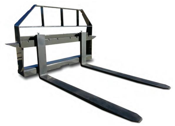
Anyone that owns a skid steer should have a set of forks on hand. Forks are ideal for lifting pallets, loading lumber or just about anything else. Our forks are 1-1/4 inches thick, 4 inches wide and 42 inches long. They are completely heat treated and rated to carry 2,800 lbs. We put a step on both sides of our frames so the operator can easily climb into the cab. Euro Style and John Deere mounts are available.
