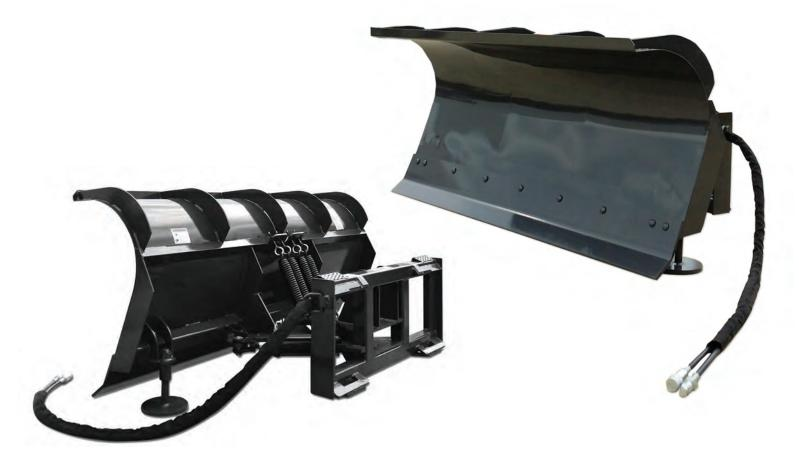
Our X-treme Snow Plow allows you to efficiently clear driveways and parking lots. Easily angle the plow from within your cab, using the  $3" \times 6"$  hydraulic cylinder. The top of the plow is rolled to keep the snow from coming back towards the cab. It's 1/2" bolt on cutting edge and adjustable snow shoes are standard.
