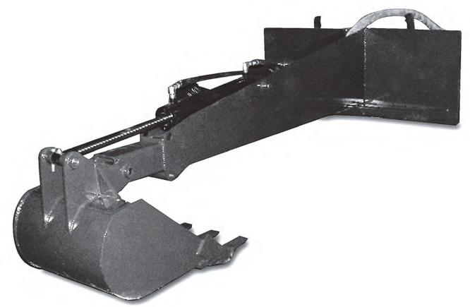
Our X-treme Stiff Arm Backhoe is an excellent tool for digging ditches, removing stumps and digging footings. With the option of adding a thumb, you can move logs, chunks of cement and most anything else. Buckets come in sizes of 8", 12", 16", 20" and 24". The bucket is powered by an American made  $3" \times 16"$  cylinder. With 7' of digging depth and 14,000 lbs. of ripping force, it is an aggressive digging machine.
