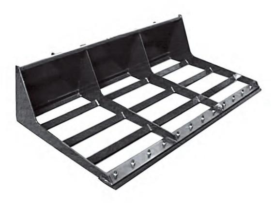
Our land leveler is 72" wide and used to cultivate, grade, cut, and mainly level land. This attachment is not designed to transfer large amounts of dirt. The land leveler is specifically used for leveling jobs such as dirt roads and gravel driveways.
