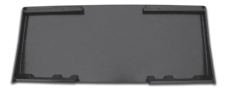
With the CID Universal Skid Steer Quick Attach plate, you can easily convert your existing attachment to the universal skid steer hook up. Simply weld or bolt the quick attach plate to the implement you wish to convert. Our standard quick attach steel plates are 1/4" thick and are solid across the back. The mounts are 1/2" thick. We can also make the steel plates thicker or thinner for different applications.
