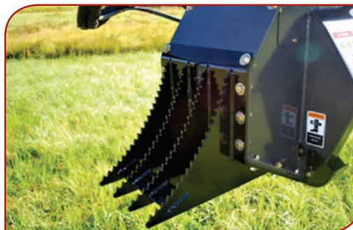
Optional thumb saddle allows operator to move obstructions out of the way without damaging the housing.
