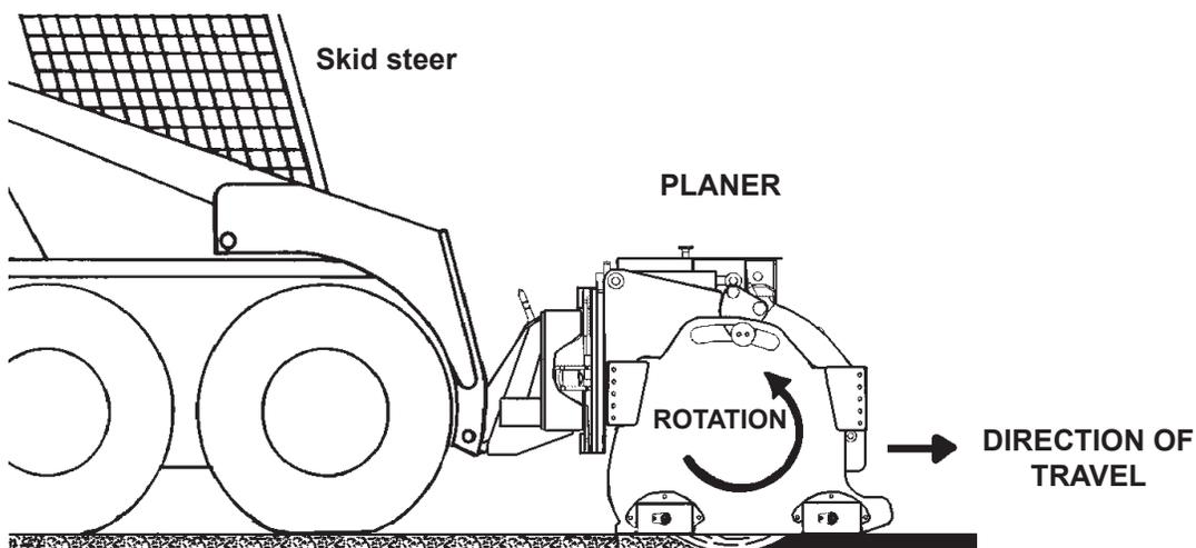
**NOTE: Mill only when the skid steer is traveling forward. Do not operate when traveling in reverse.**
