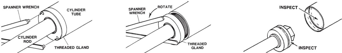
3. Remove the hex nut, piston, flat washer or spacer tube (if so equipped), and gland from the cylinder rod. If the cylinder rod is rusty, scratched, or bent, it must be replaced.
