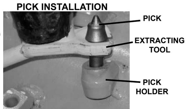
The pick is properly seated when its shoulder is against the face of the pick holder. Check to be sure the pick rotates freely.
