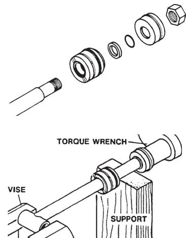
**IMPORTANT:** Do not contact the active surface of the cylinder rod with the vise. Damage to the rod could result.
