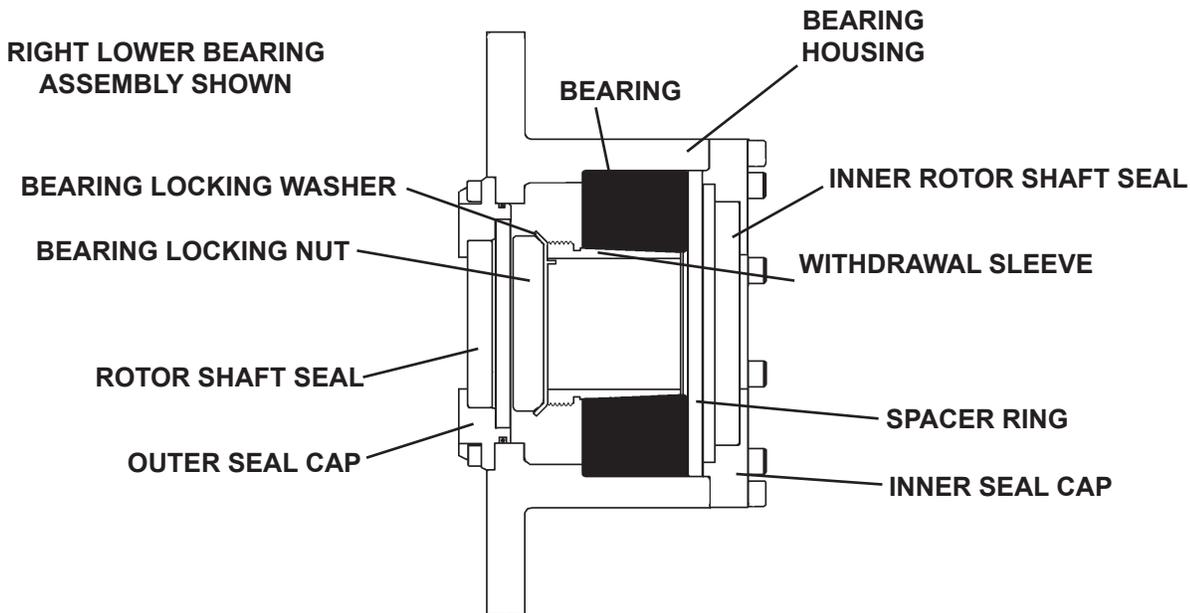
15. Apply light film of grease between the dual lips of the inner rotor shaft seals and on the rotor shaft itself where the shaft seal will be located taking extra care not to apply too much. Excessive grease will be wiped off of the seal during installation onto the rotor shaft and become trapped between the bearing inner race and the shoulder on the rotor shaft. This can wear away during operation resulting in a loose bearing.
