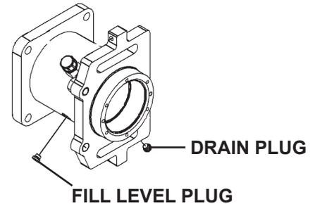
4. After ensuring that the capscrews securing the retaining seal cap to the overhung load adapter remain at 25 ft. lbs., check the gap between the retaining seal cap and the adapter housing between capscrews using a feeler gauge. This gap should be between 0.0015" and 0.010".
