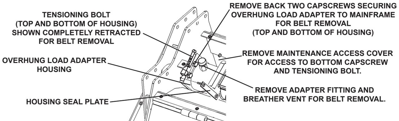
2. After testing the tension of the belt (See "**CHECKING BELT TENSION**") loosen the two cap screws on the housing seal plate (completely remove seal plate for belt removal) and the four cap screws securing the overhung load adapter to the mainframe.
