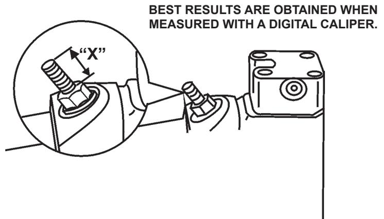
**NOTE:** These mulchers include a 6mm allen wrench and 19mm wrench to adjust the displacement screws.
