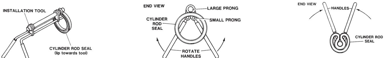
Rotate the handles on the tool around to wrap the seal around the end of the tool.
