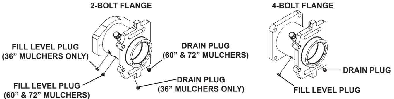
**NOTICE: The Overhung Load Adapter assembly is a sealed system. If oil level is low, check all seals for damage.**
