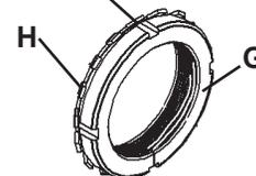
**NOTE:** Be sure the rotor is properly supported before lower bearing removal. The locking tab must be bent out of the bearing lock nut (G) prior to removal of the nut. Failure to bend out the locking tab can result in damaging the locking washer (H).
