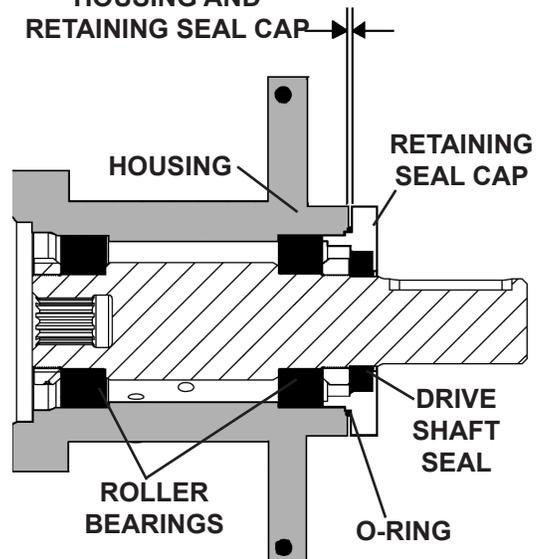
7. Remove drive shaft seal from the retaining seal cap and inspect o'ring for damage. Replace as required.
