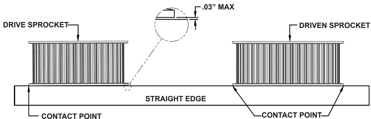
**NOTICE: Failure to align the sprockets correctly will decrease the life of the belt.**
