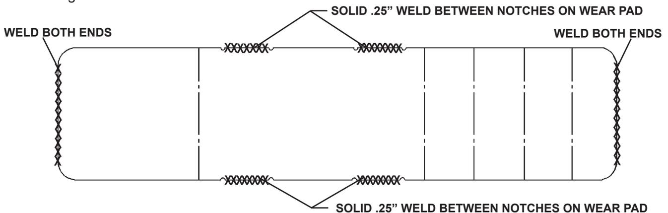
4. Prime and paint the new wear pad and skid shoe.
