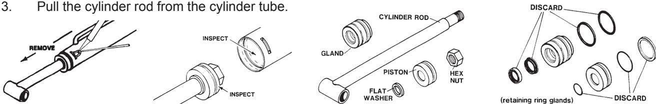
4. Inspect the piston and the bore of the cylinder tube for deep scratches or galling. If damaged, the piston and cylinder tube must be replaced.
