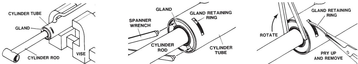
Pry up the end of the gland retaining ring with a pointed tool. Rotate the gland with a spanner wrench while removing the retaining ring. **NOTE: The gland and piston seal(s) can be pulled out and cut as they appear in the milled slot during disassembly. After cutting, pull them on out through the milled slot.**
