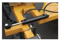
Angling capability powered by the tractor hydraulics
