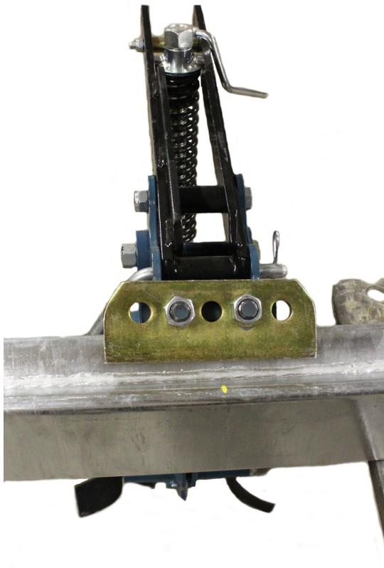
Attach the wheels to the front of the tool bar. The wheels may be located directly behind the tractor tires. They may be located in other positions as well. Some units are set up with the wheels directly in front of the outboard tillage heads. For wide machines this may not be practical. If you are working in raised beds, the wheels will typically be located in a furrow row. There is no right or wrong position for the gauge wheels!
