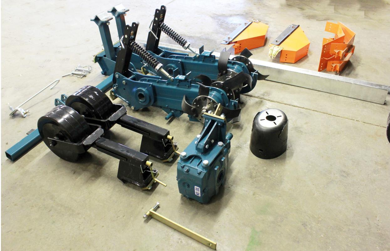
4. The frame components should be assembled first. We like to start by raising the tool bar on the fork lift so that it is at a comfortable height. You can use two saw horses or other sturdy supports to get the tool bar off the ground.
