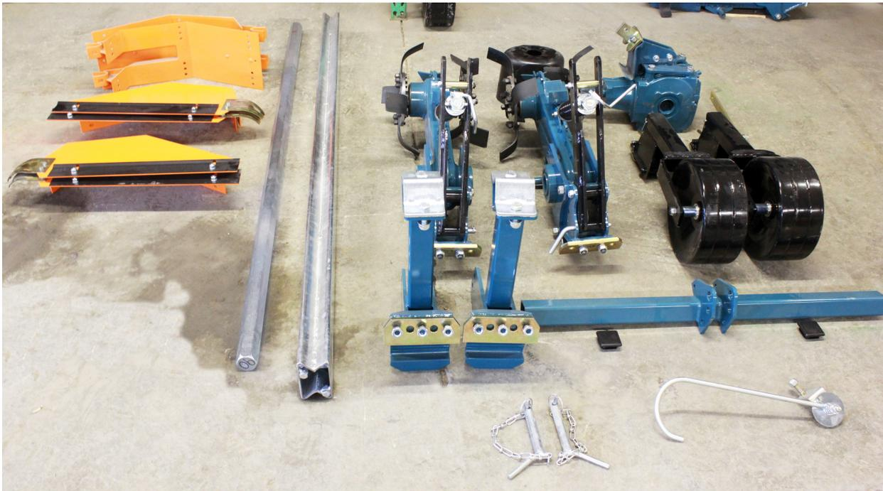
2. For this instruction sheet we are assembling a basic machine with two tillage heads. Note that your machine may have a different style three point hitch. We use A-frame style hitches on lighter FL and FLA machines, and we use wider three point hitches with two additional upright supports in addition to the two supports shown in the picture above. The components in the above picture are standard for FP and FPSR 66" and 90" wide frame packages.
