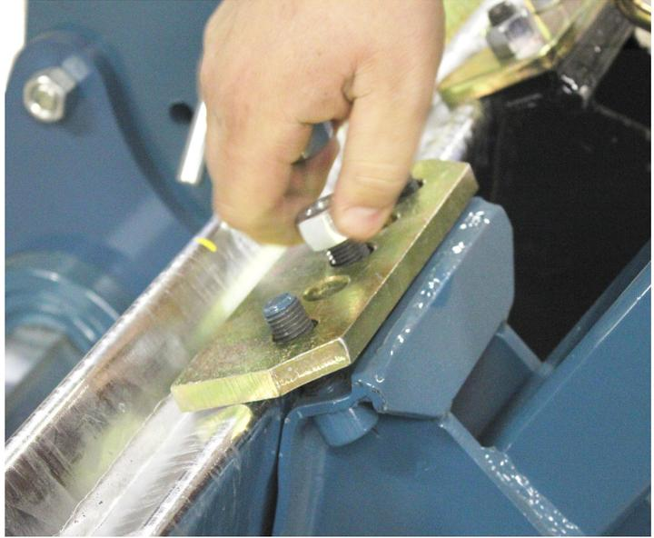
15. The completed three point hitch will resemble the picture below. The top tube has been installed and secured with clamp plates. The last step in assembling the three point hitch is to insert the square plastic caps into the top tube.
