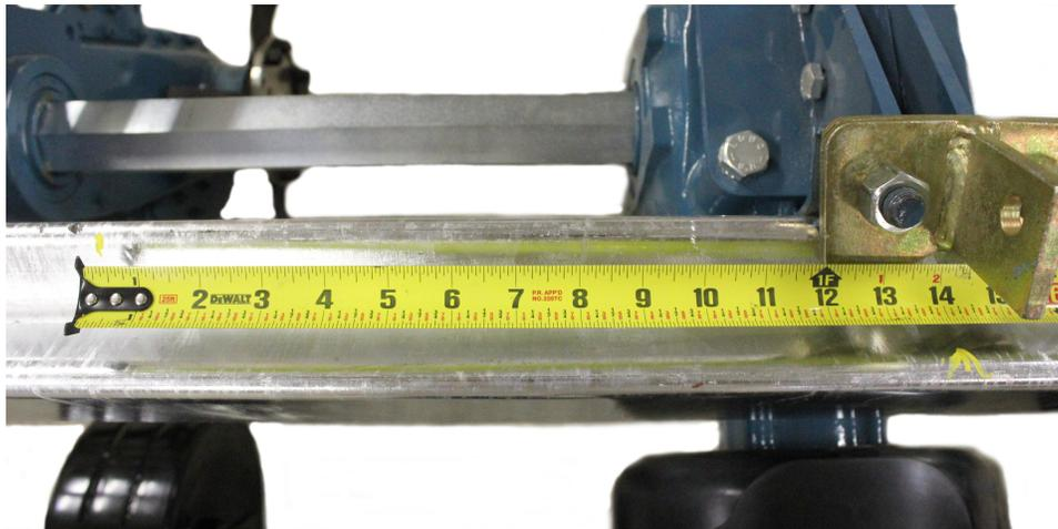
Hitch brackets are secured with clamp plates and hex nuts. Note that the tool bar design allows for elements to be moved on the tool bar as needed and front side and back side elements can slide past each other.
