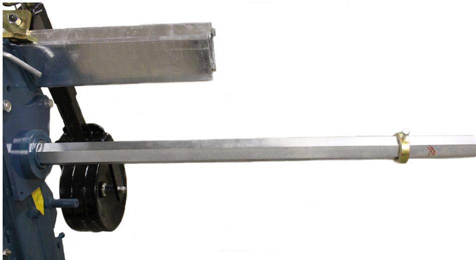
11. Once the hex drive shaft is through all of the elements and centered with the tool bar, install the hex locking collars on either side of the outboard heads. The locking collars will help prevent the hex bar from walking to the left or right during operation. Tighten the set screw in the collar firmly against the hex shaft.
