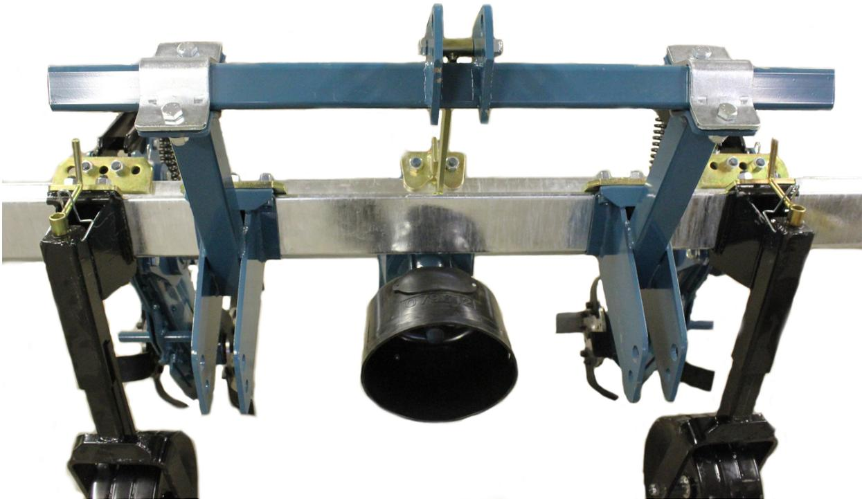
16. The rear view of the three point hitch (below) shows how the top hitch linkage bar is installed. In this example the linkage bar is attached to the gearbox which is the center element. In many cases a tillage head will be the center element, and the linkage bar will be attached to the tillage head, instead of the gearbox.
