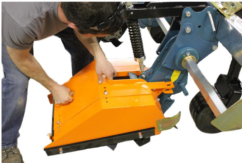
19. Insert the wedge pins and clips into the square holes in the front edge of the shielding.
