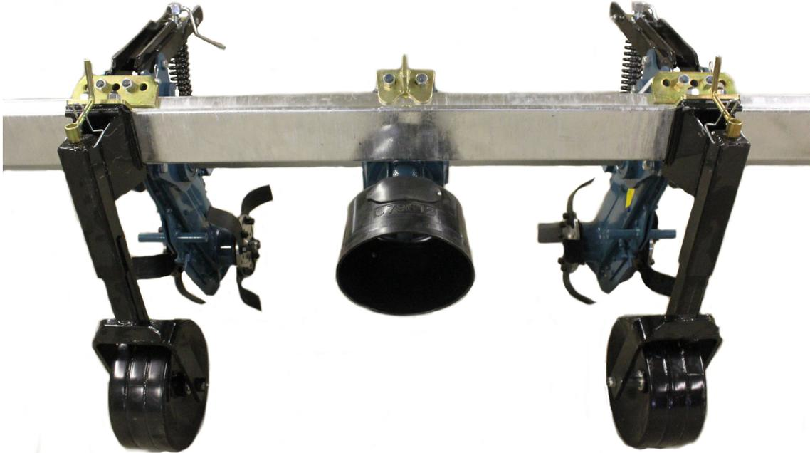
14. The three point hitch varies depending on the width of the frame. In this example the three point hitch is made up of two upright members and a top tube. Your three point hitch may be an A-frame style, or a wider version of the hitch shown in these instructions. In this example we are going to install the three point hitch uprights at 28" on center to accommodate a Cat 1 tractor hitch. Start by measuring 14" out from the centerline and mark the tool bar. Attach one upright at each point.
