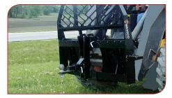
Optional features include Auger Mount, Bale Spear, & 2" Trailer Receiver Hitch
