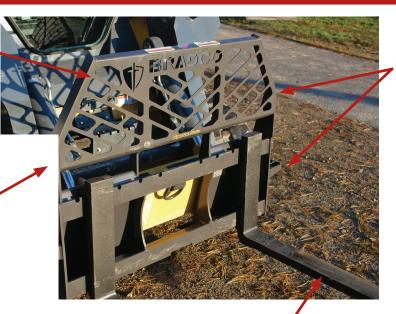
Angled side corners and a step on both sides for easy and safe entrance in and out of loader
