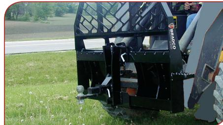
Optional features include Auger Mount, Bale Spear, & 2" Trailer Receiver Hitch
