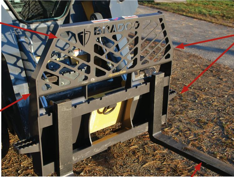
Angled side corners and a step on both sides for easy and safe entrance in and out of loader
