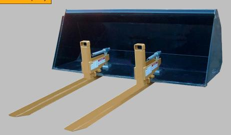
BF SERIES CLAMP-ON BUCKET FORKS mount easily in seconds to most loader buckets without using tools. Available in 1000 lb., 2000 lb., 3000 lb., 4000 lb., and 6000 lb. capacities. Slidable handle allows forks to be mounted in most positions on the bucket, such as next to the side or back of the bucket. Forks are equipped with handles for ease in mounting and handling. Forks have a safety rating of two times the stated capacity.
