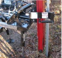
Two standard stabilizer legs offer flexibility to drive posts on uneven terrain.
