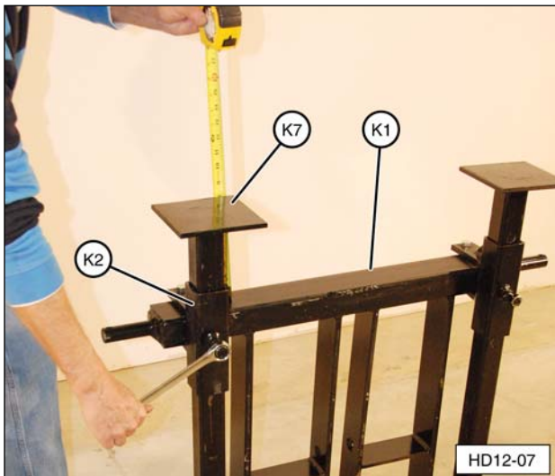
(K1) Three-Point Hitch Weldment. (K2) Leg Bracket. (K7) Stabilizer Leg.
