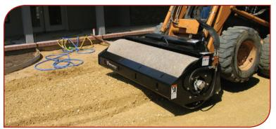
The Bradco Vibratory Roller, by Paladin, is skid steer compatible. The rollers are designed to follow ground contours for even compaction.
