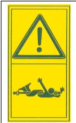
2. Indicates that it is dangerous to touch the Cardan shaft. For all other information regarding the Cardan shaft, see the use-and-maintenance booklet specifically for the Cardan shaft which, together with this manual, makes up the documentation on safety, use and maintenance of the machine.
