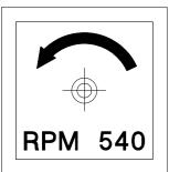
17) Shows the direction of rotation of the power takeoff and the maximum number of revolutions.
