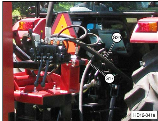
(G17) Hydraulic Supply Hose. (G20) Hydraulic Return Hose.
