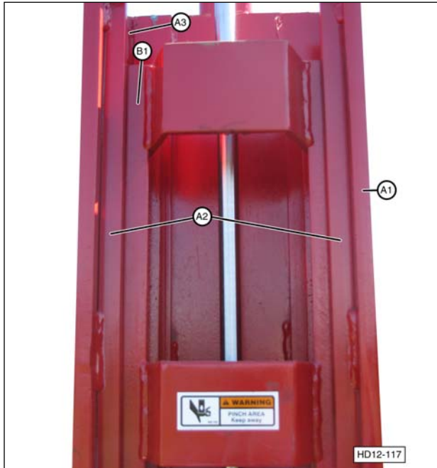
(A1) Drive Ram (A2) Guide Bar (A3) Guide Bar (B1) Main Carriage Channel.
