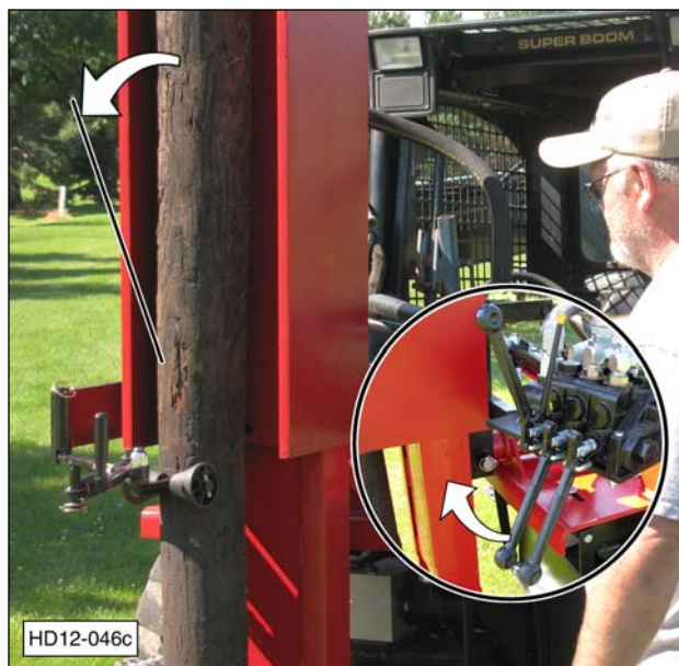
Tilt Top of Drive Ram Away From Tractor.
