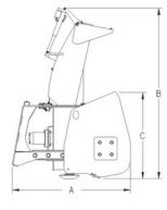
Carrier Specifications: lift capacities <9,500 lbs operating weight <11,000 lbs
