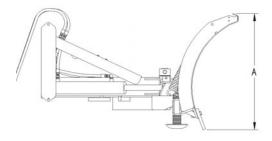
IMPORTANT: All replacement hydraulic hoses and fittings must have a minimum rated working pressure of 4000 psi. Hoses and hydraulic couplers from the attachment to the loader are included for skid-steer only.
